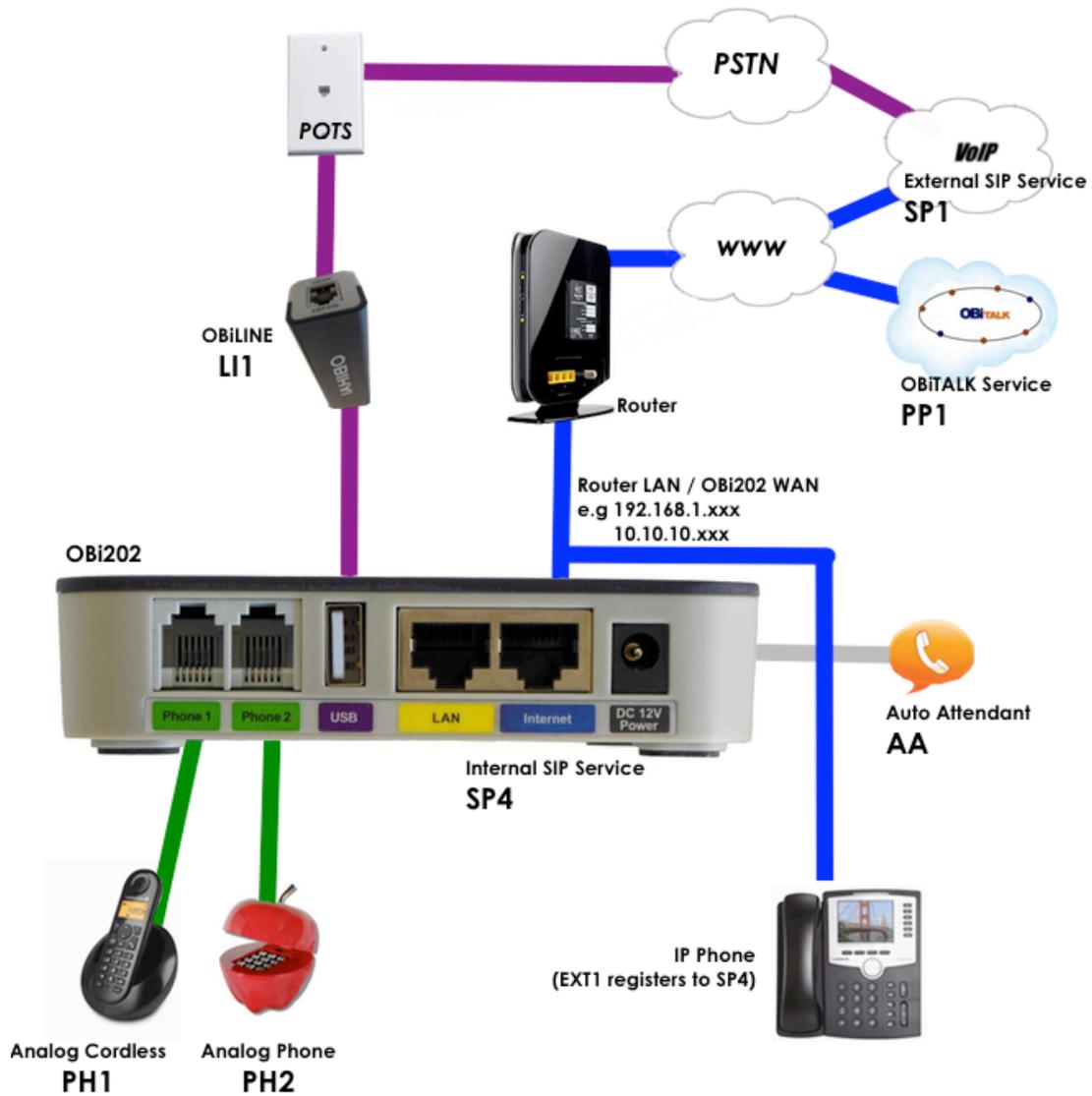
We're now going to use the OBi device as the SIP Proxy Server for the IP phone attached to router's switch port so it sits on the same flat network as all other devices.
