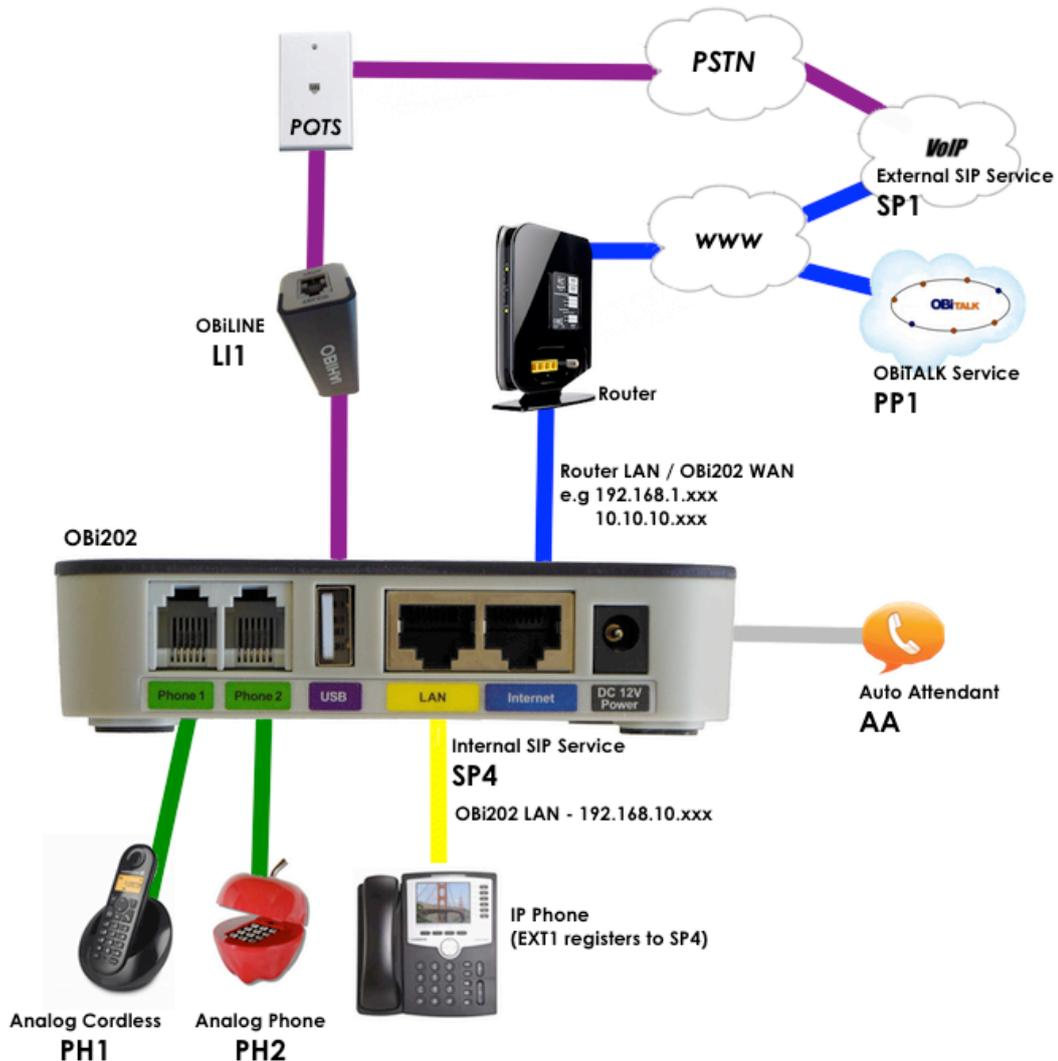
We're now going to use the OBi device as the SIP Proxy Server for the IP phone attached to the OBi's LAN-facing port. This way the IP phone registers to the OBi and can use any service configured on the OBi.
